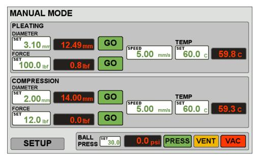
In this screen the operator can enter all setpoints for pleating and compression (diameter, force, actuation speed, temperature), as well as balloon pressure and vacuum.
