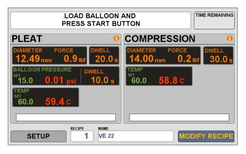
This screenshot shows recipe number 1, which is labelled as VE 22. The setpoint for balloon pressure is 15 psi, the setpoints for pleating and compression station temperature are both 60°C, and the dwell times for pleating and compression are 20 and 30 s, respectively. Vacuum will begin 10 seconds after the start of pleating. This screen also shows the current diameter and force readings for both pleating and compression stations.
