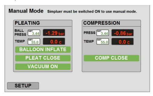
In this screen the operator can enter setpoints for balloon pressure, compression actuation pressure, pleating and compression station temperatures, and toggle vacuum, balloon inflation, and pleating and compression station actuation.
