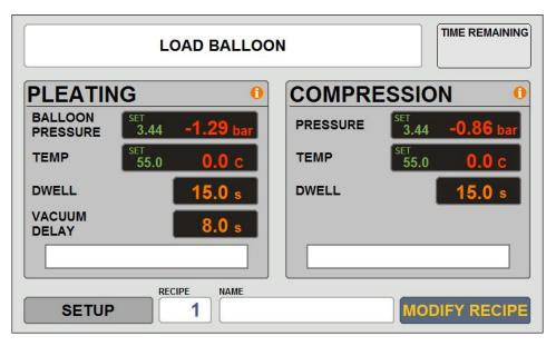
This screenshot shows recipe number 1, which in this case is left unnamed. The setpoints for balloon pressure and compression station actuation pressure are both 3.44 bar, the setpoints for pleating and compression station temperature are both 55°C, and the dwell times for pleating and compression are both 15 s. Vacuum will begin 8 seconds after the start of pleating.
