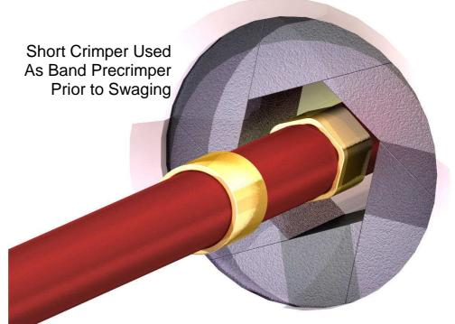
The model GPC is a hand-actuated crimper with a handle and a mechanical closed-stop. The closed-stop screw may be used to set the crimp diameter. To set the diameter, typically the operator inserts a gage pin of the desired size, then adjusts the stop screw until the jaws touch the pin.
