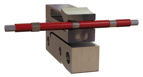
With a fixed actuation frequency, the product feed rate controls how many times the die contacts the band. The slower the feed rate, the smaller the deformation size per actuation and the better the resulting surface finish. The band is typically deformed by the die 1,000 times.
