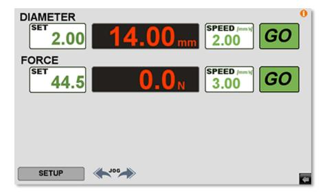
In this screen, the operator can type setpoint values and command the machine functions of diameter and force.
