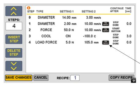
On "Load Force" and "Load Speed" steps, the "Step Options" button allows users to turn the powerfeed function on/off
