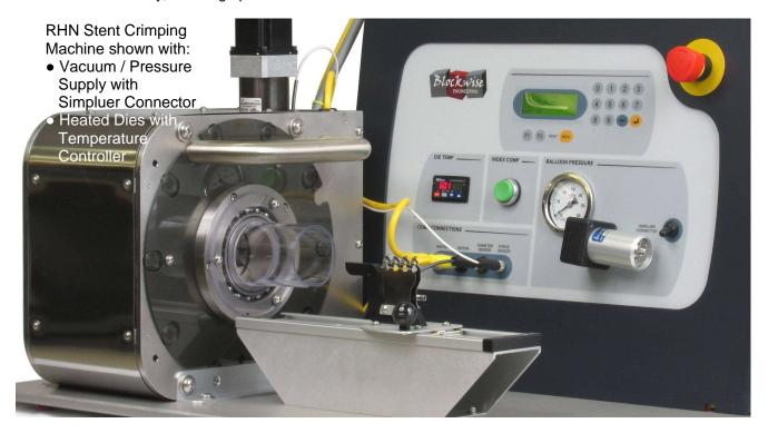
A **stepper motor** provides power to open and close the compression station. An integrated encoder measures the diameter of the opening. A **force transducer** measures the actuating force, which is proportional to the radial compression force.
