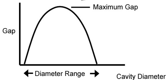
**Blockwise's J-Crimp™ and 2-Crimp™ compression station** eliminates that tradeoff, and provides a very small die-to-die gap at any opening diameter. By using J-shaped dies hinged opposite from the working surfaces, and curving the working surfaces in a specific shape, the die-to-die gap is made very small at all opening diameters.
