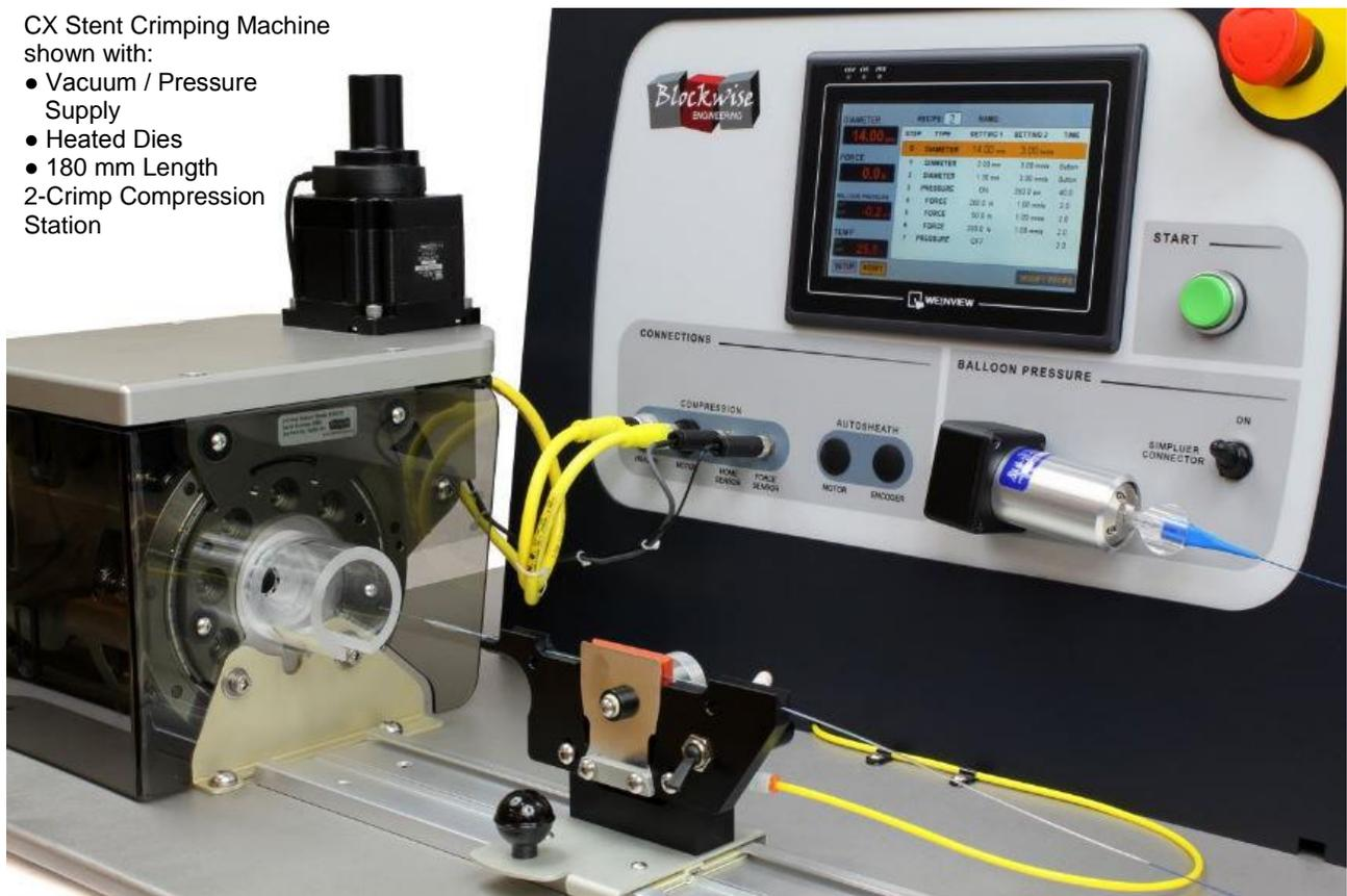
A **stepper motor** provides power to open and close the compression station. An integrated encoder measures the diameter of the opening. A **force transducer** measures the actuating force, which is proportional to the radial compression force.
