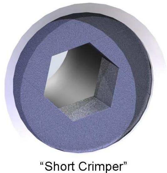
Because the length of the dies is only 6.4 mm (0.25 inch) on the model GPC, the compression force is concentrated in a small area and the pressures can be high. Dies are made from hardened stainless steel. The mechanism provides a precise center opening even at very small diameters.
