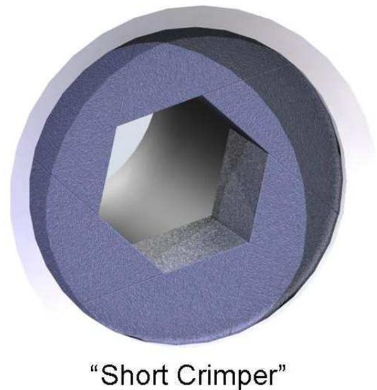
Because the length of the dies is only 6.4 mm (0.25 inch) on the model GPC, the compression force is concentrated in a small area and the pressures can be high. Dies are made from hardened stainless steel.
