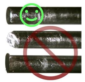
When preparing a stepped pushrod, the above advice is still applicable to the end of the larger diameter rod. However, for the end of the smaller, mandrel part of the rod, a rounded end is ideal. A rounded tip will help the smaller portion of the rod to easily slip into the stent while it is compressed.
