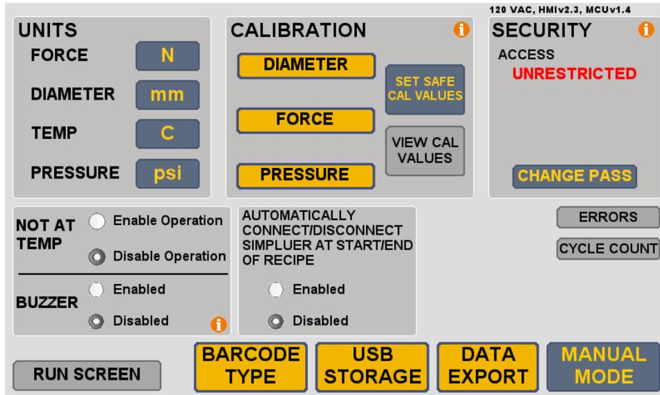
The SETUP screen allows changing of parameters that apply to the whole machine (not just one recipe), and allows access to other functions such as:
