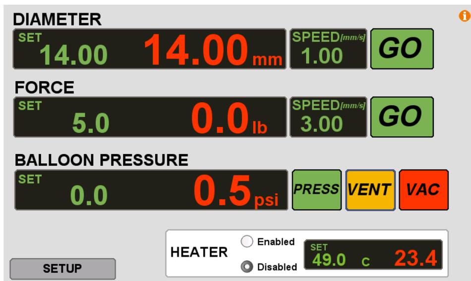
In this screen the operator can type setpoint values and command the machine functions of diameter, force, pressure, and temperature.
