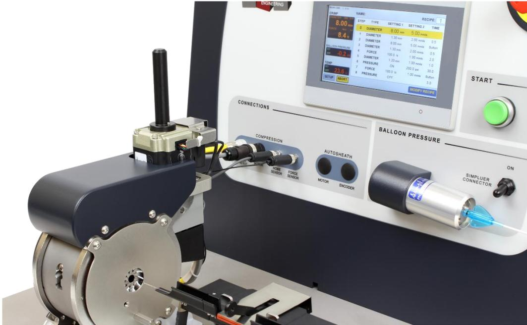
**RUN SCREEN** – The most-used screen. It displays live indications of diameter, force, temperature, pressure and the selected recipe’s number, name and steps.
